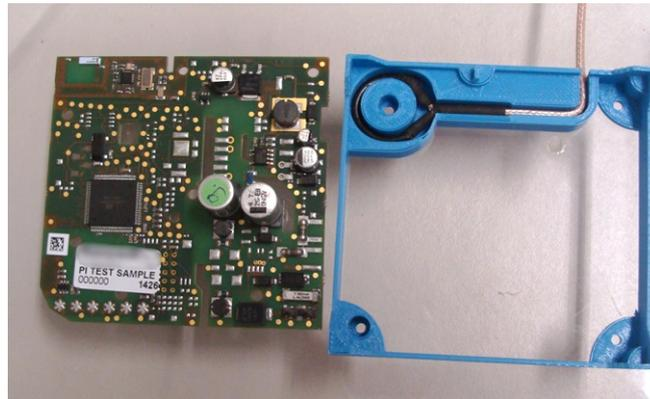
The picture shows an 868MHz PCB with an Ethertronics Savvi loop antenna in the upper left corner. On the right is the loop probe in a 3D-printed test fixture.
