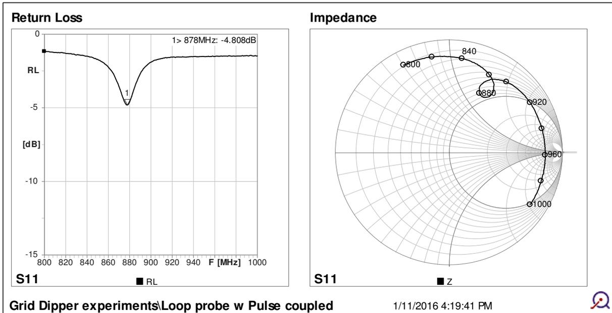
The Smith chart shows that the probe by itself is inductive (near the upper edge of the top half circle), but that the antenna pulls the impedance toward the center (50 Ohms) at its resonance.
